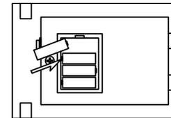
Insert 4 AA batteries into the battery compartment on the inside of the door.
