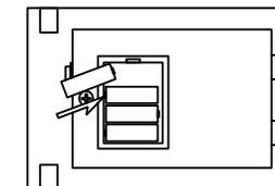
Insert 4 AA batteries into the battery compartment on the inside of the door.
