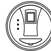
The red light flashes and indicates that the battery has a low charge and needs to be replaced.
