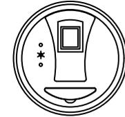
2. The green light flashes, a 'beep' sounds and all fingerprints are deleted. The safe is now in the factory state and can be opened with any finger.
