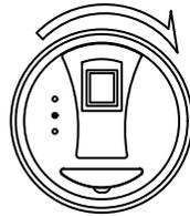
2. The green light illuminates. Turn the lock ring within 6 seconds to open.
