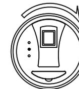
The green light illuminates. Turn the lock ring within 6 seconds to open.
